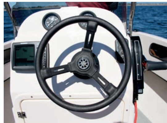
The well designed console has space for a decent-sized flush-mounted display and the controls are pleasingly light, not stiff like some installations
