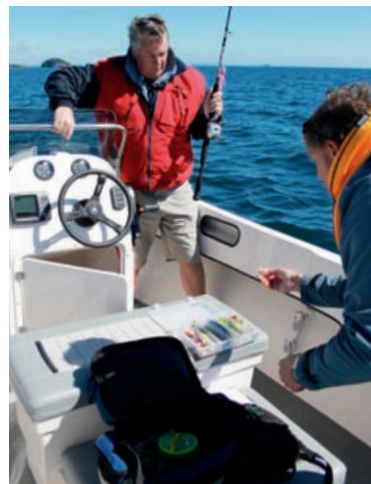
A bench-style helm seat with under-squab stowage and two removable seat bins
